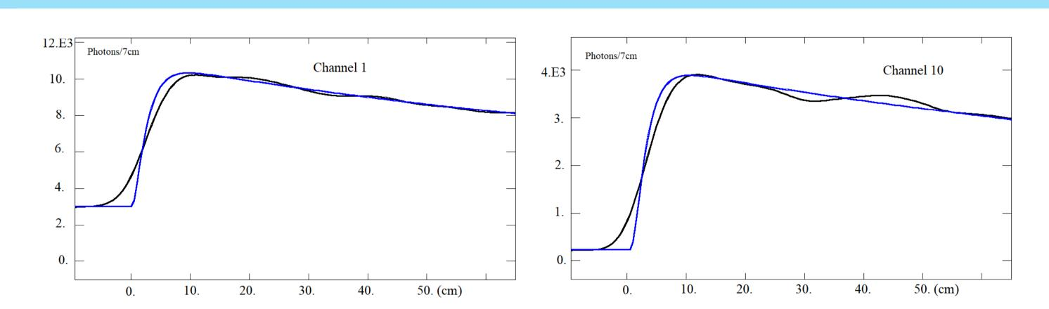
When the barrier region is shorter than our resolution the laser beam sees a kind of step function. The measured signals will all, to some extent display the leading part of our detection response function. The figure shows the scattered signals in two channels compared to the non convoluted input data.
