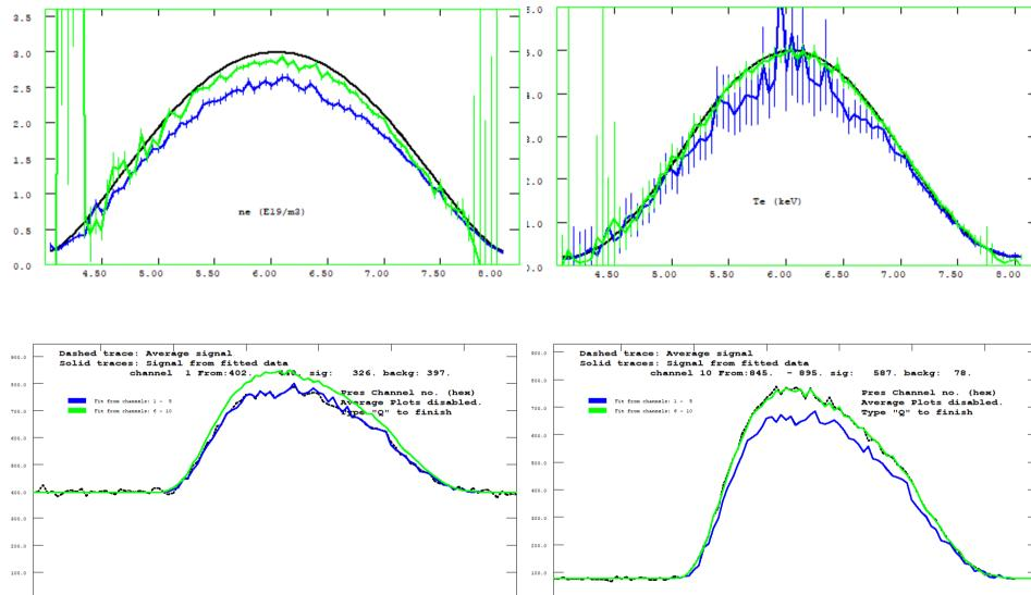
At low temperature (<6-7 keV) the spectra from each of the two wavelengths barely overlap. This allows us to make two independent fits to the data. The fit shown is based on an average of 10 measurements.
