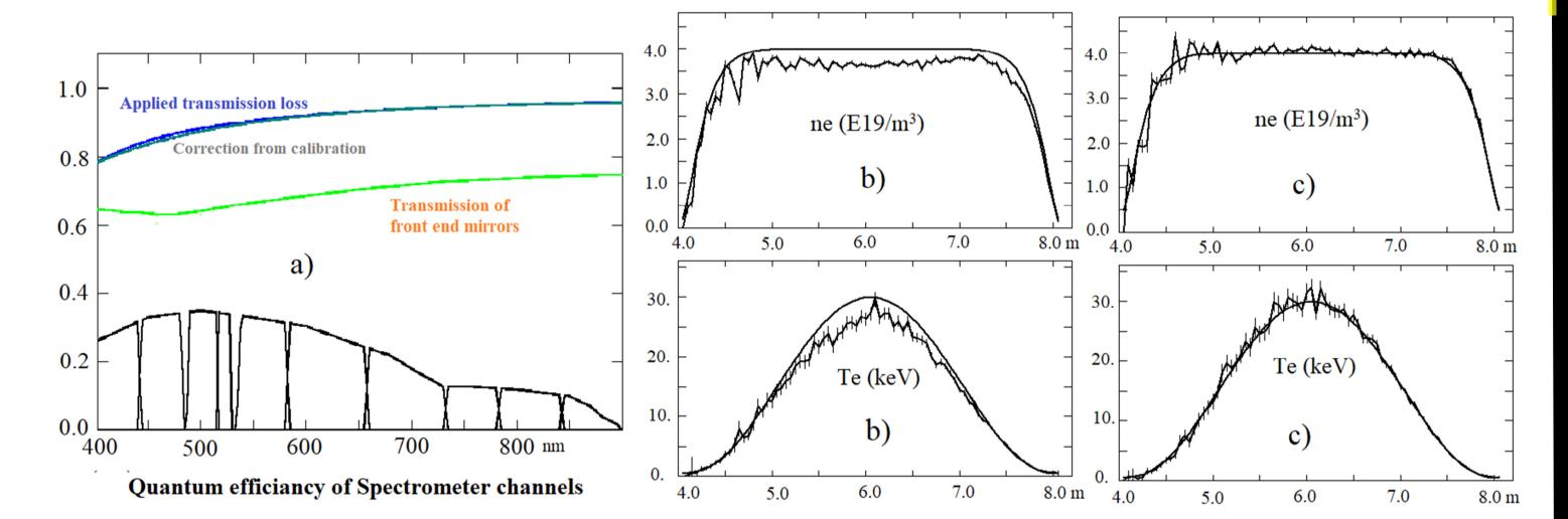
In the simulations we introduce an artificial change of the transmission. The change is illustrated in (a) "Applied transmission loss". Fitting these new data with the "old" transmission yields the results shown in (b), showing the fit relative to the input data.
